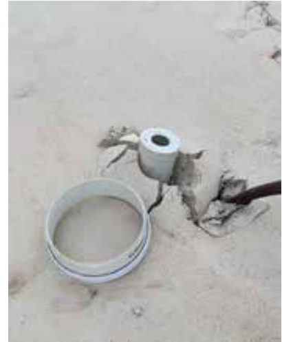
Fig. 1 Sifter and PVC pipe used to collect sand samples
